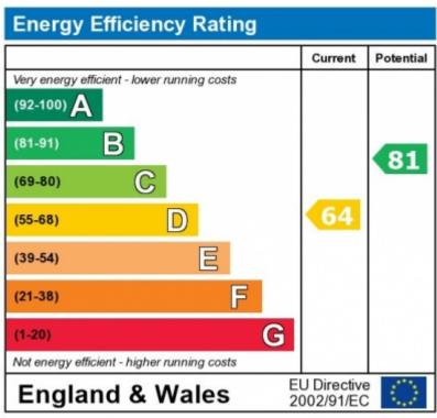
The energy efficiency rating is a measure of the overall efficiency of a home. The higher the rating the more energy
